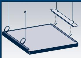
**Step 1:** Prefix the suspension wire on the ceiling and to the joining bar, roughly adjusting the height as necessary.
