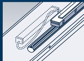
**Step 3:** Insert the luminaire into the raft.
