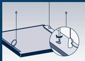
**Step 2:** Pre install the screws on the raft, lift it up and fix it to the joining bar.
