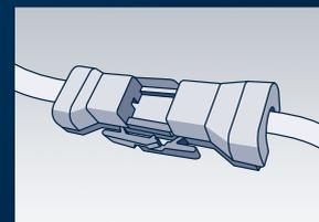
**Step 4:** Connect all luminaires electrically with the pre fixed connector.
