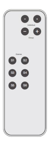
Point the handset at the detector and press a button. The beam angle is quite narrow, so accurate aiming is important.
