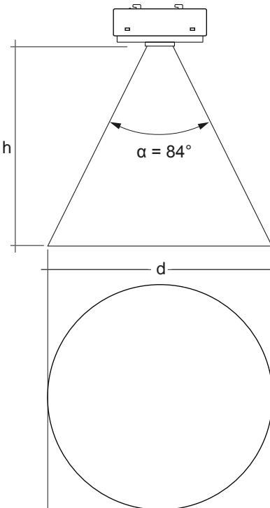
Example for light and motion detection area at height of 1.7 m:
